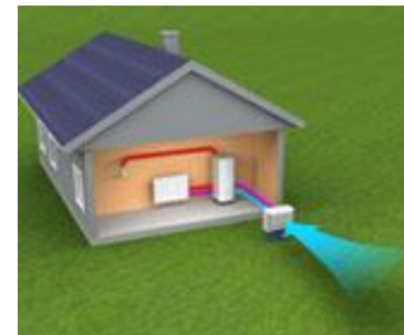
Air Source Heat Pump
