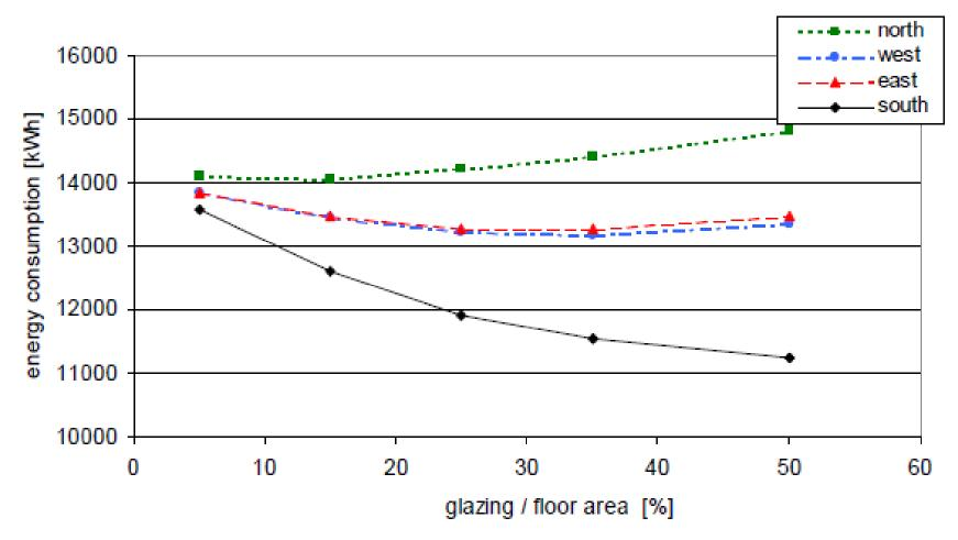
Energy consumption kWh/year (space + water heating) V's Glazing ratio.
