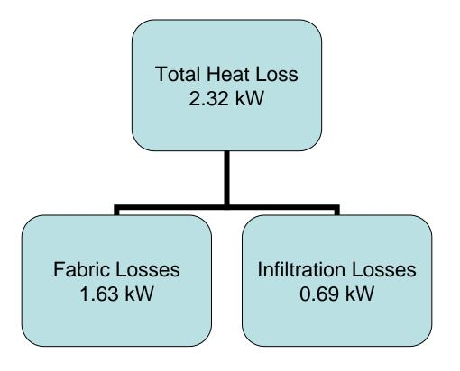
In this example infiltration accounts for 30% of the heat loss
