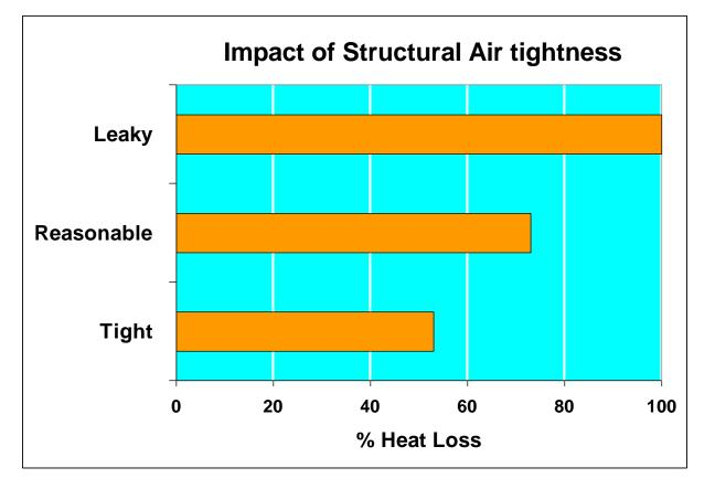
Improving structural air tightness from 0.9 ac/h to 0.03 ac/h reduces the heat loss by 47%, all other factors remaining constant.
